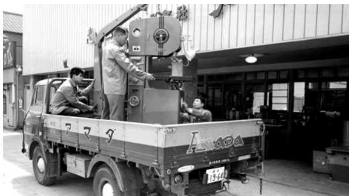
Vertical Contour Bandsaw on demonstration at a customer's site.
