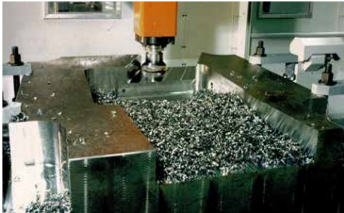
Dry machining with HSC: High-speed machining entirely without cooling lubricant – what started out as an experiment at the beginning of the 21 st century has become a symbol of resource-saving manufacturing.
