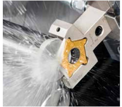
PENTA-IQ-GRIP tool with dovetail clamping mechanism provides high pressure coolant supply in two directions.
