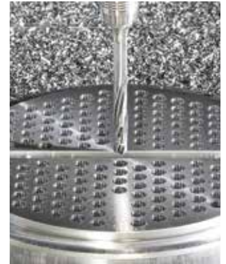
Helical flutes with variable helix angle in a LOGIQCAM drill body improve the dynamic behavior of the drill and increase the drilling depth to eight drill diameters.
