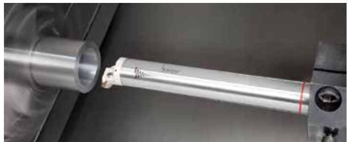
Anti-vibration boring bars WHISPERLINE enable stable cutting with the overhang up to fourteen diameters.
