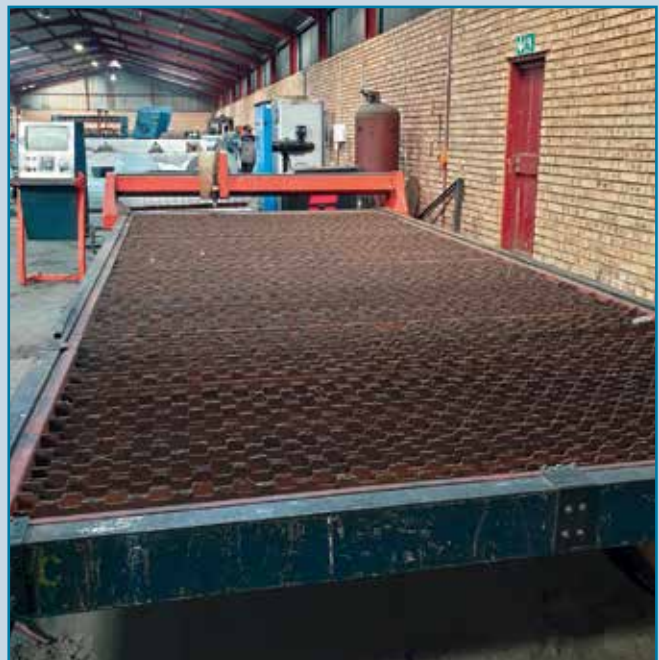
6000 x 2500 High Definition Plasma Cutter with a Hypertherm HSD130 Plasma Source
