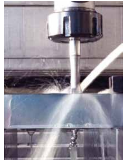
NORIS STABIL UNI HSS-PS TiCN in machining situation through hole: Chips are evacuated in the cutting direction.
