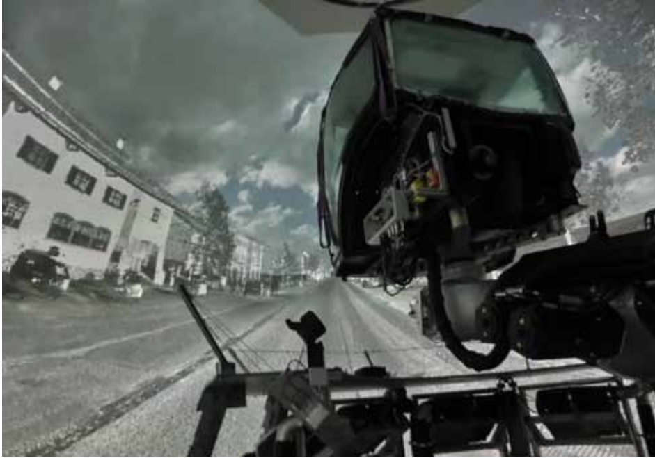
Virtual vehicle development is becoming increasingly important. Researchers at Fraunhofer are offering a system that takes into account realistic environmental influences like road surface, weather and driving maneuvers in driving simulations. © Fraunhofer ITWM
